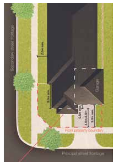
Porches, verandahs, pergolas, eaves, fascia and gutters can encroach by up to 1.5m
